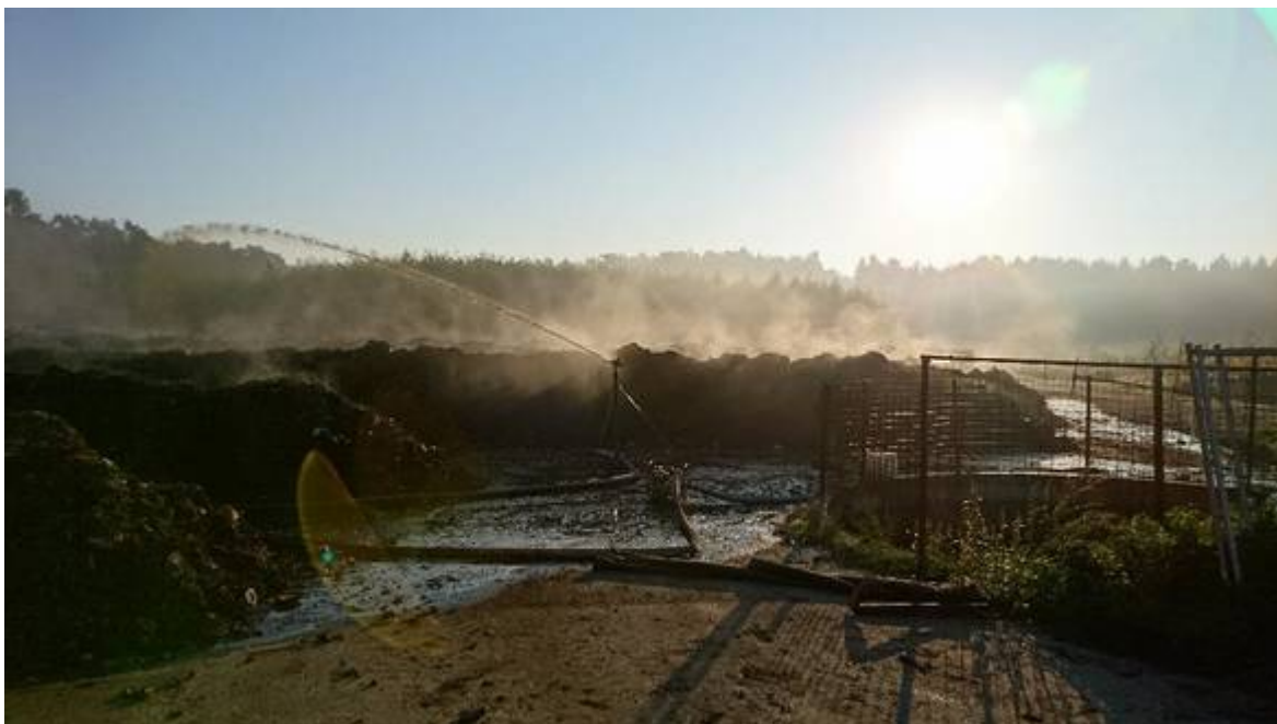
Adjusting or spraying with waste water for proper moisture content (40 -50%)
